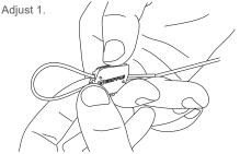
Ensure a minimum 75 mm of tail wire exit the hanger.
