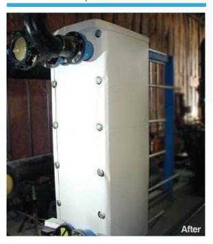
HexWrap® is a unique, flexible insulation blanket specifically designed for Plate & Frame Heat Exchangers. It consists of a flexible, pre-fit outer jacket bonded to either open-cell or closed-cell foam insulation. HexWrap® is easily installed and is adjustable if you expand your heat exchanger. Service temperature ranges from -70°F to +350°F and intermittent up to 400°F. HexWrap® also has low smoke and flame ratings, designed to be
